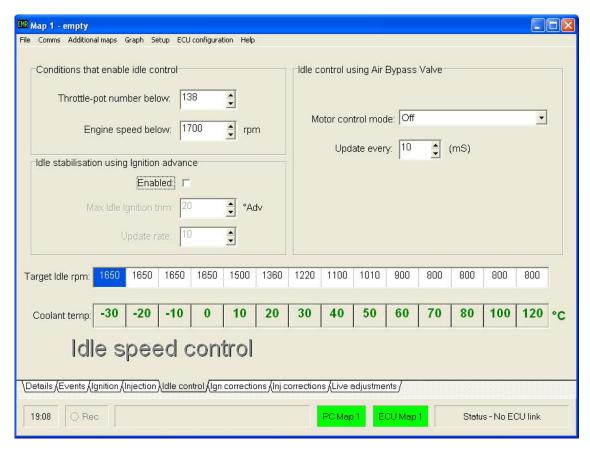
Note that your "Throttle-pot number below" within the "Conditions that enable idle control" area of the screen will be unique to your installation so **do not** set it to match the above screen shot. After making the changes, re-program the map/ECU. Now select the "Live Adjustments" screen (F8) and start the engine.
