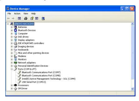
Click on the Ports Icon to reveal all currently in use ports on your PC. With the USB-serial adapter connected it should appear in the list. In the above example the Port identified is Com13. Select that port when opening the Emerald software.
